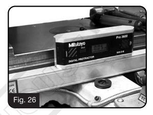
When mounting the reader head if necessary pack the reader head (Fig. 27) so that it travels in line and square to the scale to avoid any damage to the scale. Testing for parallel can be done by either a dial indicator or a precision level. (Fig. 26) The cover must be fitted (Fig. 28)
