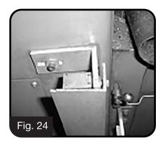
The "Z" axis scale should be installed on the side of the column ensuring that the open side of the scale is away from direct swarf and coolant and that the travel is in the right direction "-" towards the spindle and "+" away from the spindle. The bracket (Fig. 22) is mounted off the knee, and around the scale (Fig 23) to allow for the cover (Fig.24) to protect the scale, where excessive coolant & swarf are present.
