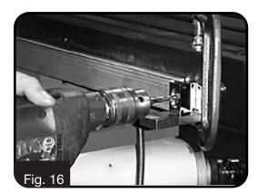
When the scale is mounted then fix the reader head to the saddle, if necessary packing the head to ensure that it is parallel and in line with the scales. (Remove the grey packing between the reader head and scale which allows for the correct clearance and holds the reader head parallel to the scale.) (Fig. 16)
