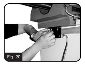
After the scale is aligned to the axis, then drill and tap the saddle to suit the bracket provided and mount the bracket ensuring that the reader head is sitting correctly so that when the reader head is attached it will be square and parallel to the scale. (Fig. 20)
