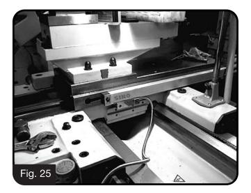
The scale should be mounted ensuring that it is parallel and square to the slide. (Fig. 25)
