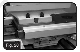
The longitudinal scale should be mounted on the back of the Lathe (Fig. 29) with the open side of the scale facing down and must be parallel to the bed. The reader head is mounted to the saddle (Fig. 30) via the brackets provided. Some modification may be required for some lathes. Covers should be mounted over the slides. (Fig 30)
